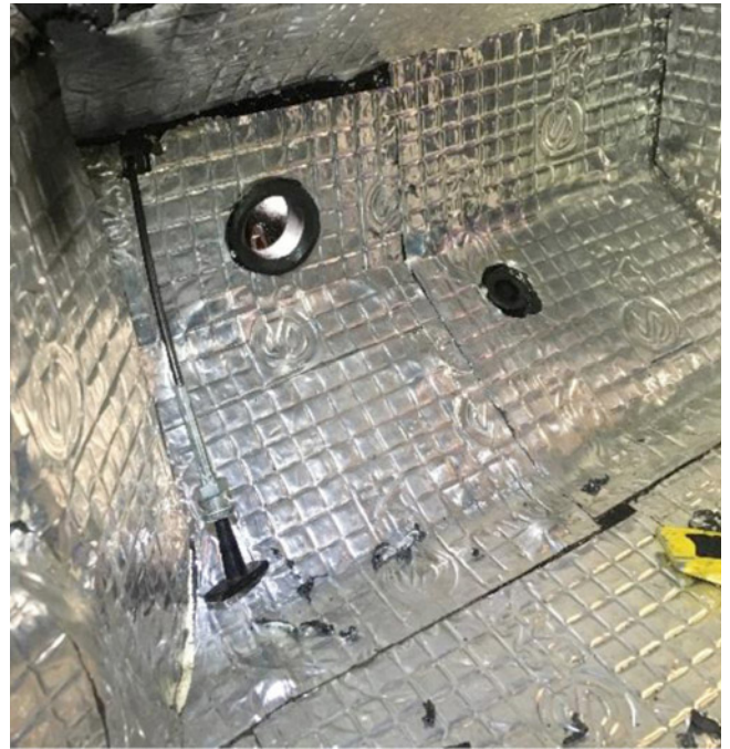
Above: Passenger footwell, showing Silent Coat (or Dynamat) style insulation with holes drilled and grommet fitted.
