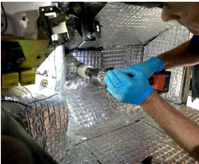
Above: Passenger footwell, showing Silent Coat (or Dynamat) style insulation with holes drilled and grommet fitted.
